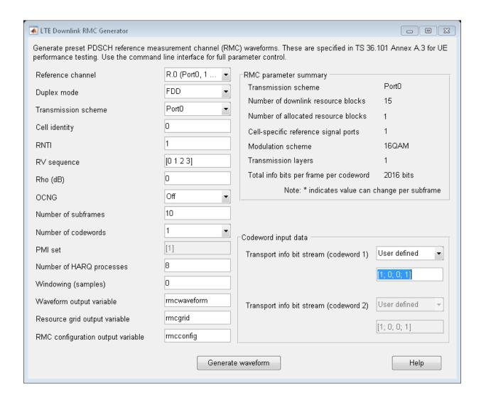
You can use the user interface to generate the default waveform or adjust default settings prior to waveform generation.
