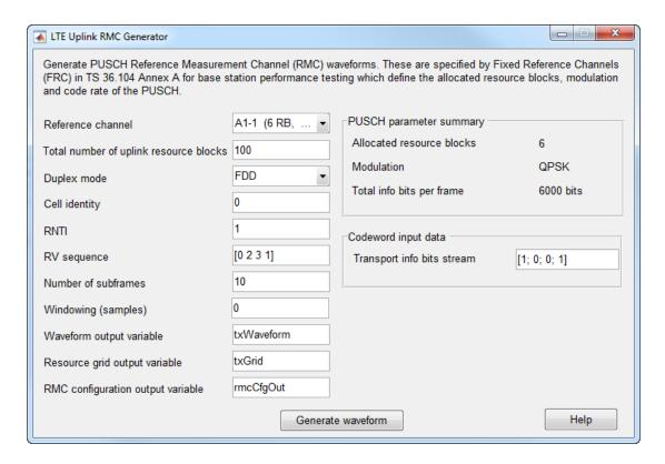
Click **Generate waveform** and the txWaveform, txGrid, and rmcCfgOut variables appear in the MATLAB Workspace browser.
