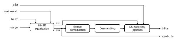
If the resource element grid across all possible EPDCCH antenna ports is input, the function extracts all EPDCCH resource elements and performs EPDCCH decoding for all possible EPDCCH candidate locations. The function assumes the input symbols were already equalized. Each EPDCCH candidate is descrambled individually during EPDCCH search.
