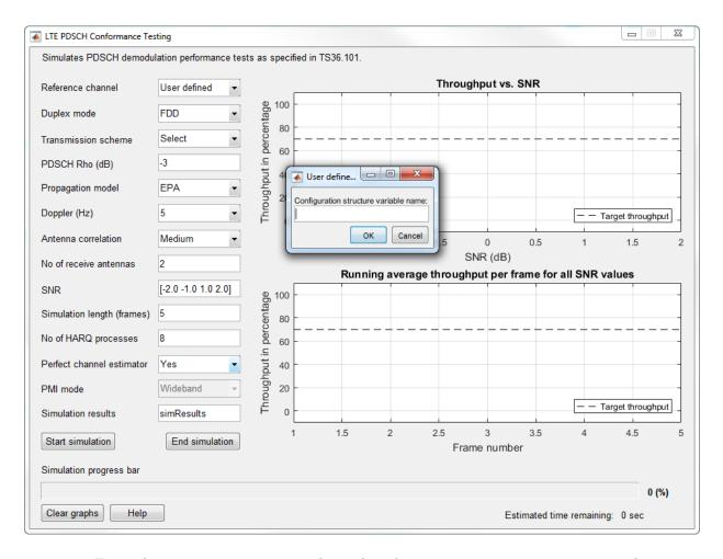
Enter the custom measurement channel configuration structure name, CMC, in the prompt. When the simulation is run this user defined configuration will be run.
