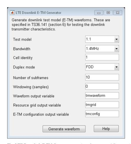
The LTE Downlink E-TM Generator user interface opens. Adjust settings and output variable names as desired.
