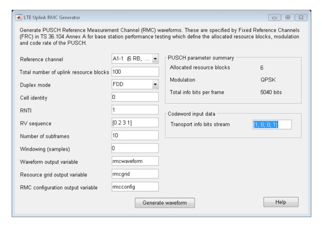
Use the user interface to generate the default waveform or adjust default settings prior to waveform generation.
