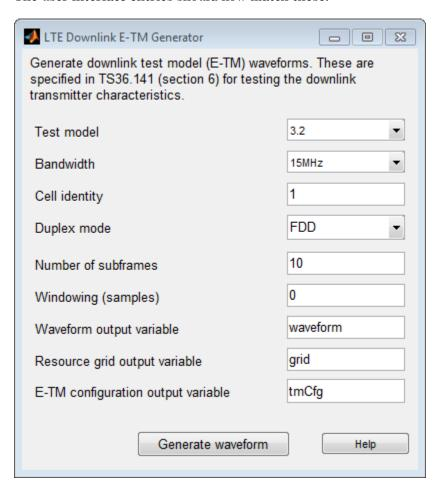
Click **Generate waveform** and waveform, grid, and tmCfg variables now appear in the MATLAB Workspace browser.
