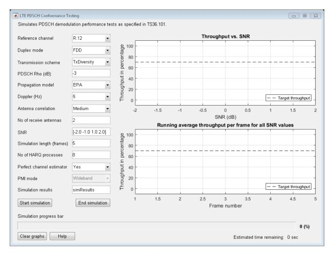
The LTE PDSCH Conformance Testing user interface opens.
